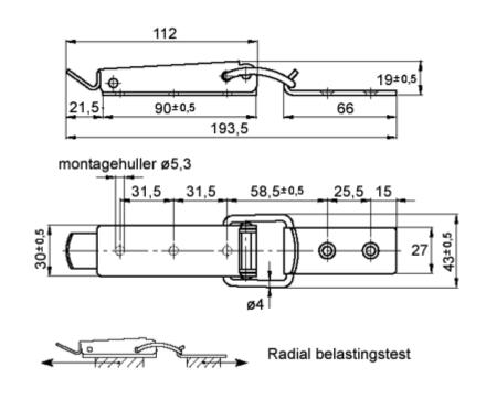
$\begin{array}{l} \text{Max load (N)} &= 2000 \\ \text{Ultimate strength (N)} &= 4000 \end{array}$
